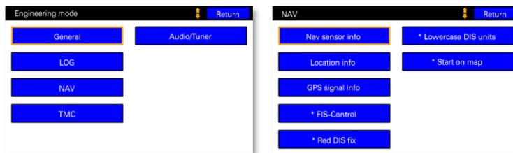
Toggles for new features can be found under the Engineering Mode's "NAV" menu. Within each menu configurable features are prefixed with an asterisk.
