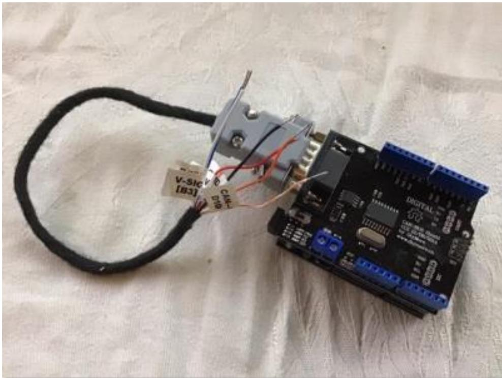
Note however that the Arduino's inputs are still only 5v, and the reverse gear and speed signals as 12v. You will need to buffer the input signals so as not to damage the Arduino:
